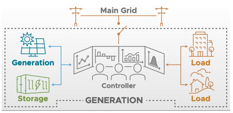
Figure 1. Microgrid components (dashed box) and switch connection to the main grid (top)
